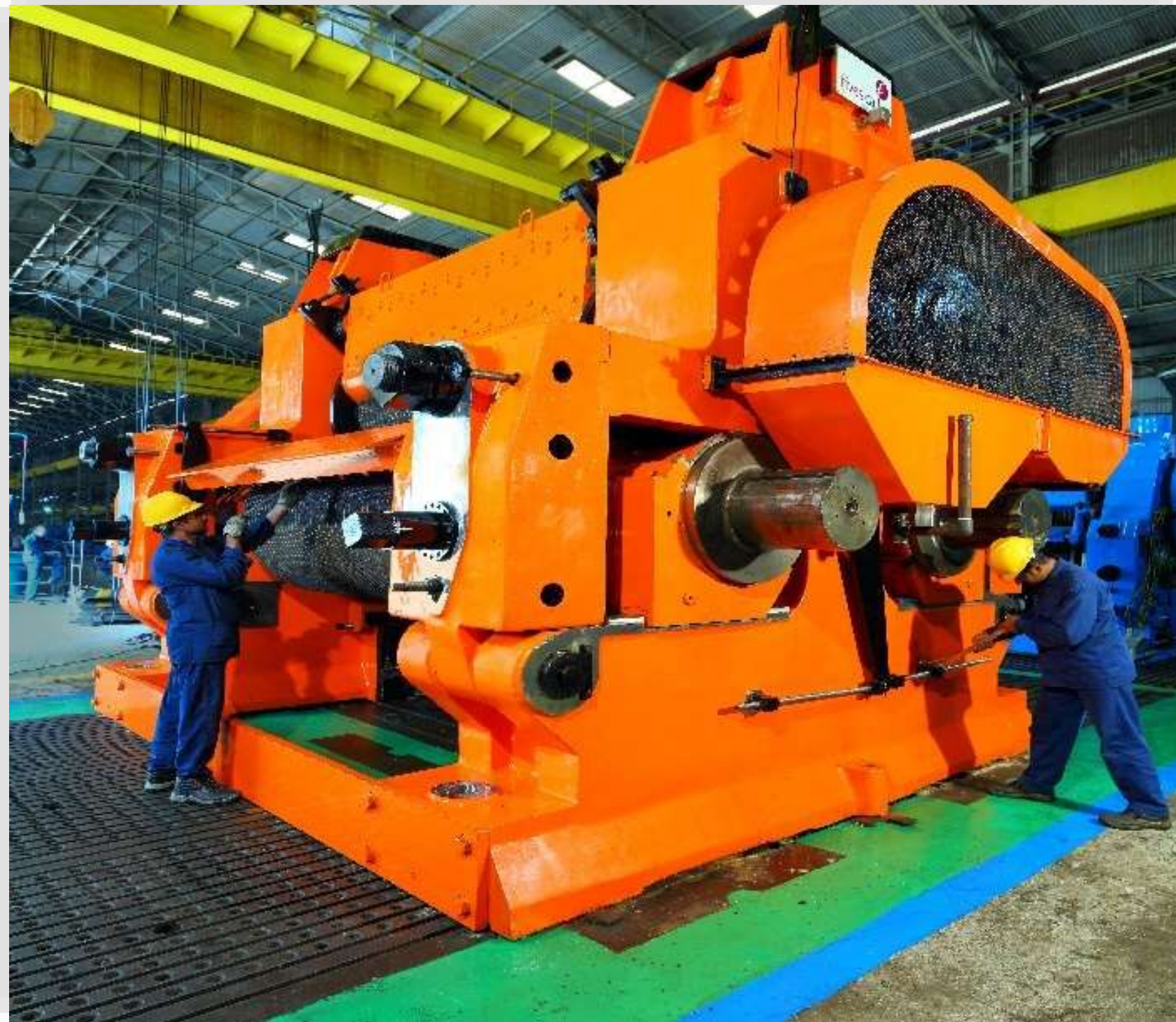
50" x 100" 4-Roll Mill designed by Fives Cail France
